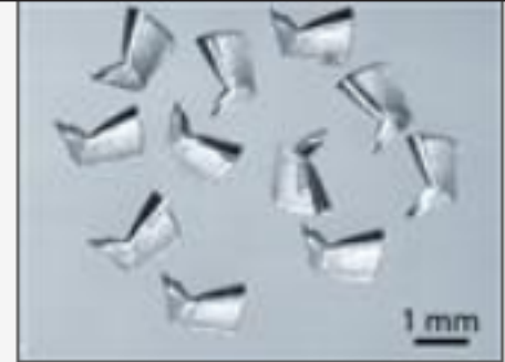
Here are chips from the same material produced when the tool was used in modulated machining.
